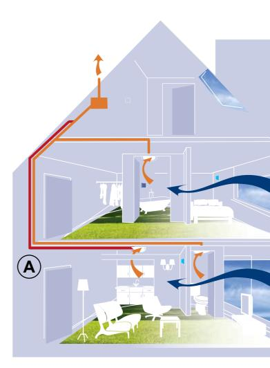
**Fig A** - Illustrates a typical "System 3" or central extract duct layout, focusing on the 'Best Practice' that the toilet extract is separate to, or positioned in line between the kitchen extract and the extract unit. iCONstant dMEV
